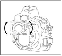
6. The 45° viewfinder can be rotated at any desired angle.
