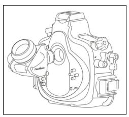
4. Align the 45° viewfinder with the viewfinder mounting ring in the display window as shown in the diagram.
